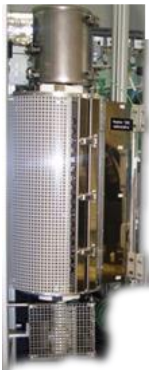
reactor with tubular furnace and insulation
